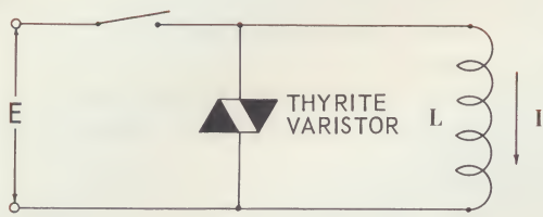
Protective Circuit FIGURE 5
